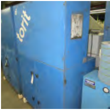
Torit Dual Cartridge Vibra-Shake Dust Collector, Model VS- 3000
