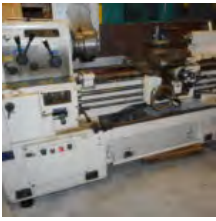
Royal / Whacheon 17" / 24" x 40" Geared Head *Inch / Metric* Gap Bed Lathe
