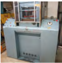
500 Ton Ferrara Hydraulic Coining/Stamping Press
