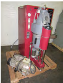
Neutec Vacuum Induction Casting Machine Model J15 1 of 2
