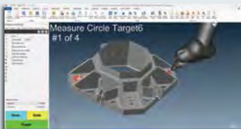
Align Part to CAD Model
