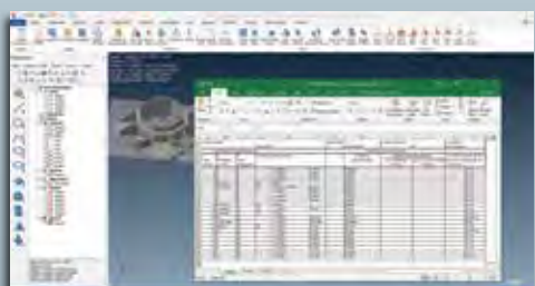
Report Part Deviations Compared to Nominal CAD
